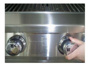
Push and turn the main, rotisserie or sear burner control knobs to the "HI" setting. Push the control knob until the burner ignites. The burner should ignite within 4 seconds (if burner does not ignite follow match lighting instructions on Page20). After the burner is lit, adjust the heat level as desired.
